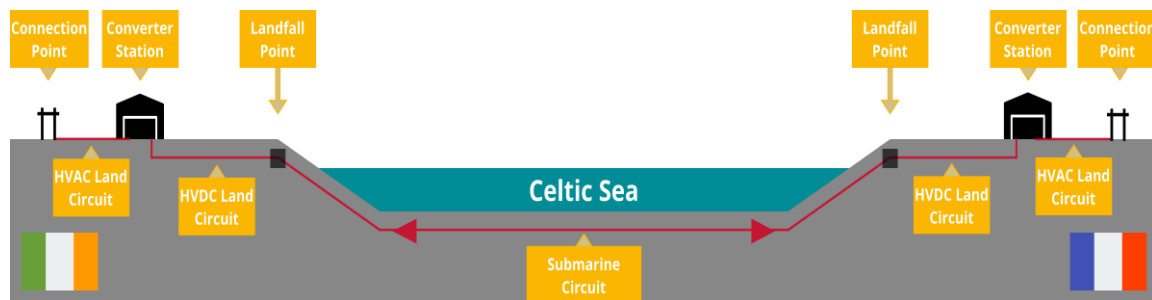
Figure 3 - Celtic Interconnector Project Elements
